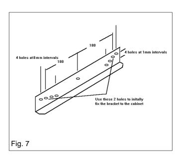
Check that the mounting brackets are level.
